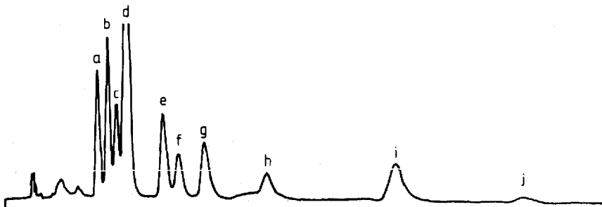
Fig. 2. Separation of adenosine nucleotides on C_{18} (Ro Sil). Conditions as in Table II. a = AMP; b = ADP; c = ATP; d = AMP( S ), ADP( \beta - S ), ATP( \gamma - S ); e = ( S_p )-ATP( \beta - S ); f = ( R_p )-ATP( \beta - S ); g = ( S_p )-ADP( \alpha - S ); h = ( S_p )-ATP( \alpha - S ); i = ( R_p )-ADP( \alpha - S ); j = ( R_p )-ATP( \alpha - S ).
